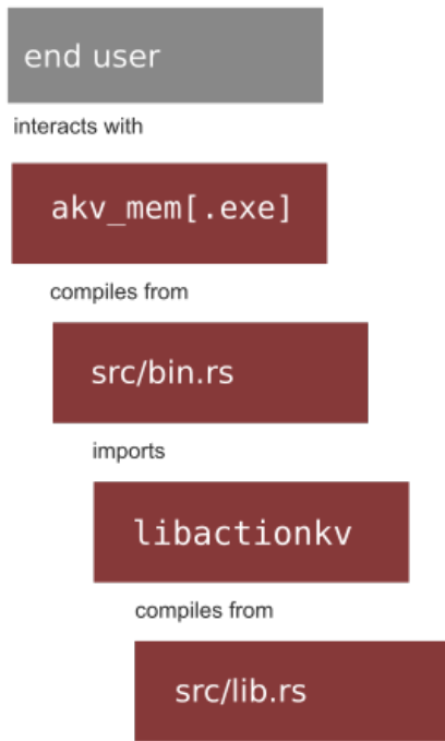
Figure 7.6. Relationship between libactionkv and other components of the project
